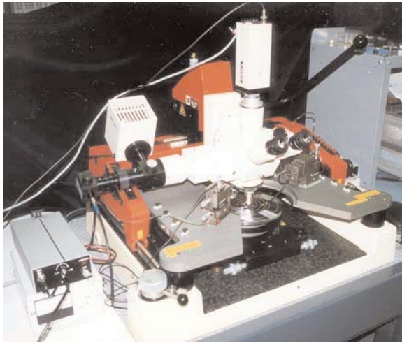
The MicroPoint laser provides deprocessing/removal of passivation and other materials for probing at the smallest sites.
